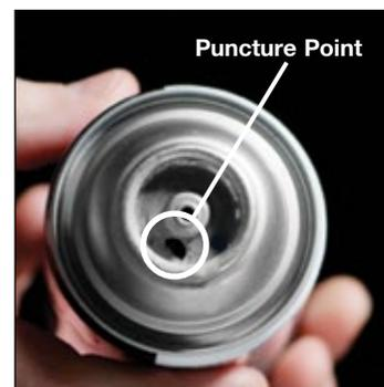
Most efficient puncture point at the dome top (rather than side) offers fast evacuation and less mess.
